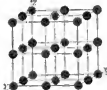
FIG. 5.—The unit cube of the NaCl-arrangement (4b, 4c). The atoms in positions 4b are shown as annuli; those in 4c as black circles. The coordinates of 4c are 0\frac{1}{2}0 ; \frac{1}{2}00 ; 00\frac{1}{2} ; \frac{1}{2}\frac{1}{2}\frac{1}{2} .
